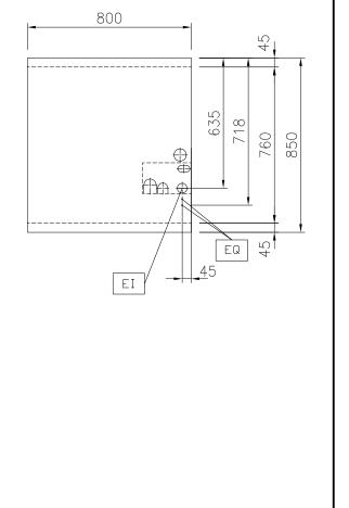
Electric Supply voltage: 400 V/3N ph/50/60 Hz Electrical power, max: 12 kW **Key Information:** 100 °C **Working Temperature MIN:** Working Temperature MAX: 450 °C External dimensions, Width: 800 mm External dimensions, Depth: 850 mm External dimensions, Height: 250 mm Net weight: 120 kg Configuration: One-Side Operated;Top Front Plates Power: 3 - 3 kW **Back Plates Power:** 3 - 3 kW Solid top usable surface 670 mm (width): Solid top usable surface 650 mm (depth):
